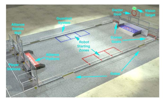
At each side of the Playing Field, two-inch wide lines of gaffers tape define three five-by-five foot areas. These areas are the Robot Starting Zones. The tape is colored red or blue, to indicate which alliance should use the Robot Starting zone. The tape is not part of the Robot Starting zone. There is a 2" white line across the center of the field between the robot starting zones.
