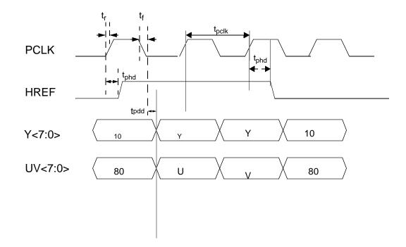
FIG 2.2 Pixel Timing
