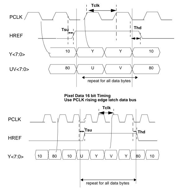
Pixel Data 8 bit Timing Use PCLK rising edge latch data bus
