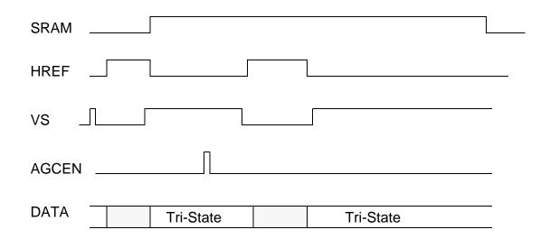
**SRAM** is internal control bit which is high means the OV7620 enter external RAM status. This is programmed by SCCB (register **27**) or power-on read-in. When **SRAM**=1, OV7620 all data bus will be tri-stated and ready to send the data. Micro-controller will send a initial signal to FPGA to reset all RAM Address block, after that, there are two method to get one frame data frame OV7620:
