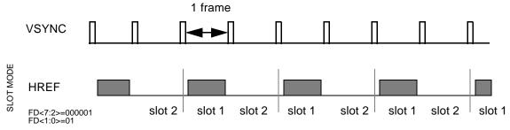
FIG 1.10 Frame Division Examples (Progressive Scan Mode)
