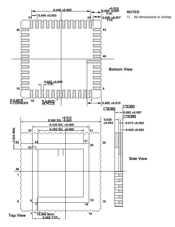
FIG 2.6 Package Mechanical Data
