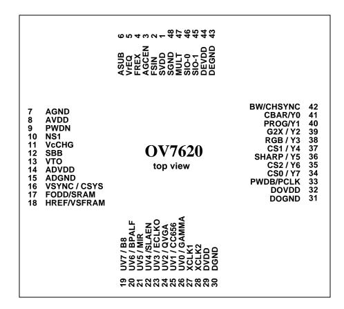
FIG 2.1 OV7620 48Pin Digital Package
