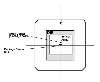
Top View FIG 2.7 OV7620 Sensor Array Location (in inches)
