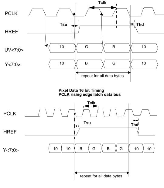
Pixel Data 8 bit Timing PCLK rising edge latch data bus
