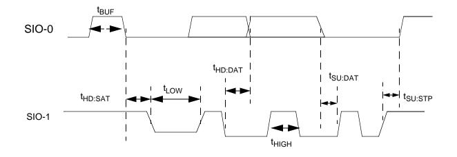
FIG 2.3 SCCB Bus Timing
