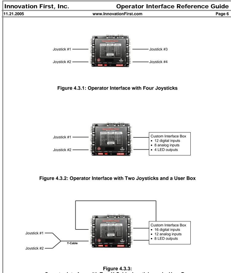
Operator Interface with Two Y-Cable Joysticks and a User Box
