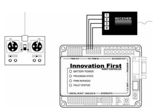
The EDU Robot Controller can use the signals from standard hobby radio-control (R/C) receivers for remote operation. In this manner a human operator can use the joysticks and switches on their standard hobby R/C transmitter to control the robot.
