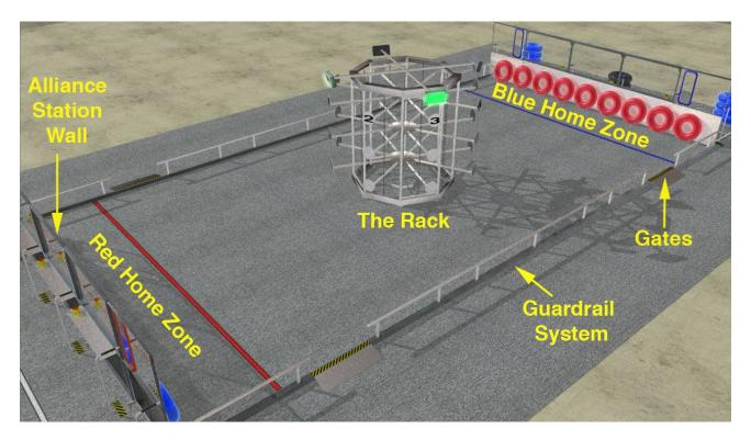
The Alliance Station Wall is 6-1/2 feet high. The entire Alliance Station Wall is 26 feet 8 inches wide, centered on the ends of the field. The wall is composed of a 3-foot high base of diamond plate aluminum topped with a 3-1/2-foot high transparent acrylic panel.
